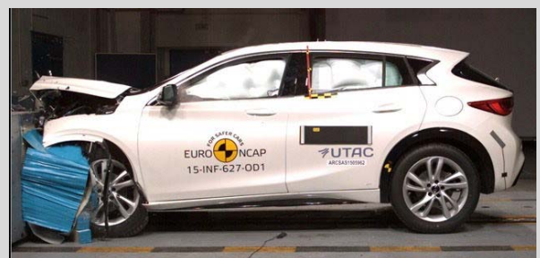
Frontal offset test at 64km/h
