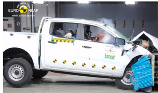
Offset crash test at 64km/h (Ford Ranger)
