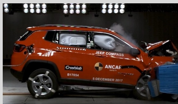
Frontal offset test at 64km/h
