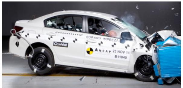
Offset crash test at 64km/h (Impreza)
