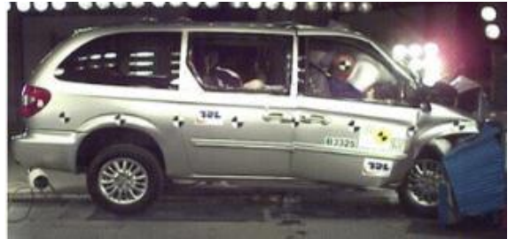
Offset crash test at 64km/hr
