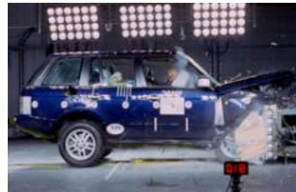
Offset crash test at 64km/hr
