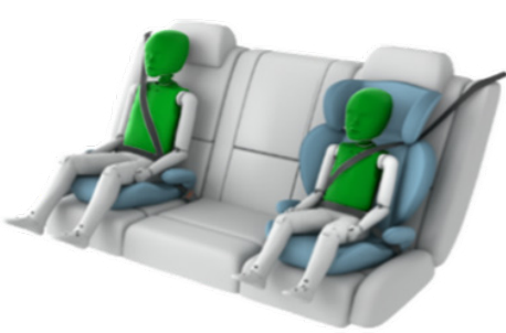
SIDE IMPACT TEST - 60km/h
