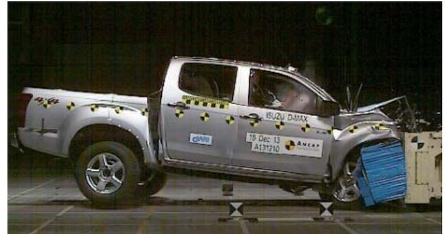
Frontal offset test at 64 km/h (D-Max utility tested by ANCAP)
