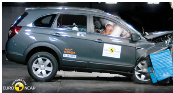
Offset crash test at 64km/h
