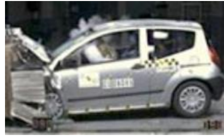
Offset crash test at 64km/hr
