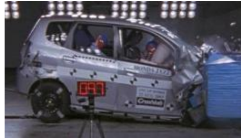
Offset crash test at 64km/hr
