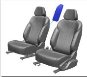
Driver's seat has a far side airbag in addition to the side airbag. Location of far side airbag is shown in the mark. 9. on page 1.
