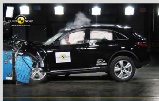
Frontal offset test at 64km/h
