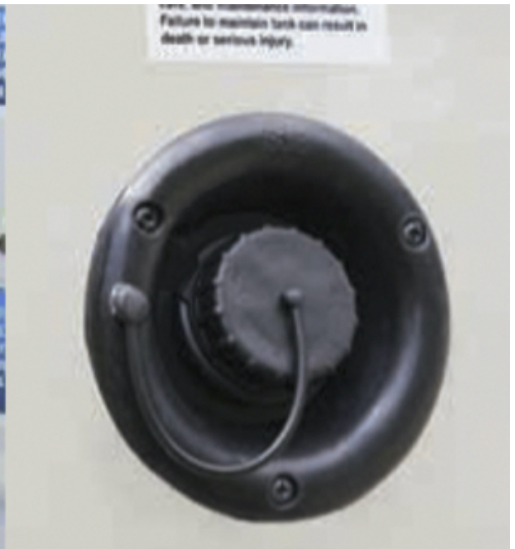
(L) Fresh water fill connection. (R) Gravity-controlled water intake.
