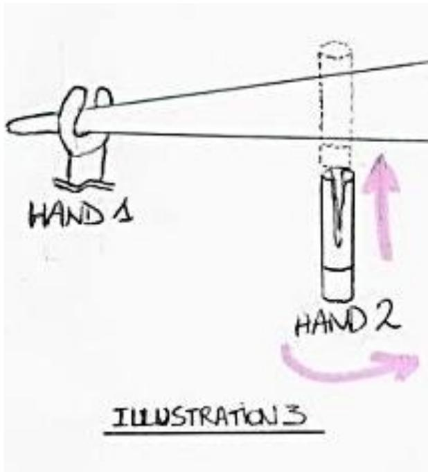
Then the cobot **puts the film in the reel** placed in the other arm. Once the film is between the two parts of the reel, the cobot starts getting the reel to turn around itself in order to **wind the plastic film onto the reel**.
