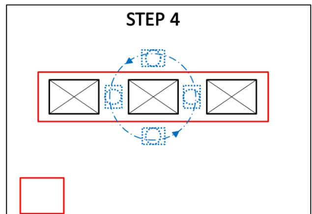
During the unfilming step, the cobot is able to **feel a tension** against its reel due to the **torque sensor** of its arm. This tension comes from the plastic film which is around the pallet. At the end of the operation, a section of the film falls down and doesn't resist to be wound. From that time the cobot **knows that there is still a precise number of rotation to do**.
