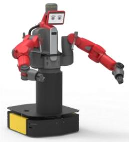
We will use a **humanoid cobot** placed on an **AGV**. We decide to equip this cobot with a **vision captor**, a **2D lidar** and intelligent sensor with TOF camera. Eventually the cobot will handle a **reel** in its right arm and have a **clamp** in its left arm.
