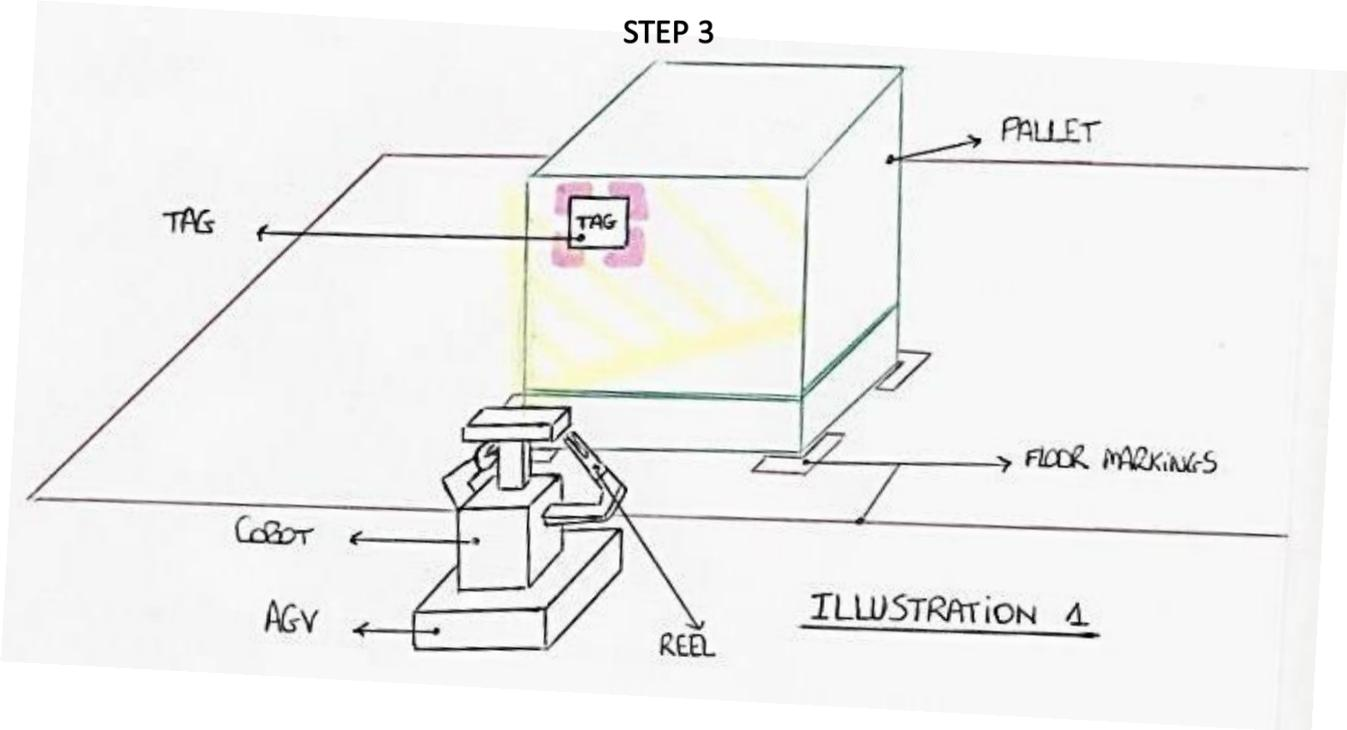
Above we can see illustration number 1 which shows how the "cobot + AGV" are getting ready to unfilm the pallet in front of them.
