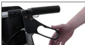
3. To unlock the brakes, pull up on the brake lever until the lock is removed.
