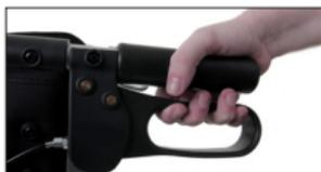
2. To lock the brakes, push down on the brake lever until it locks in place.
