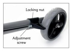
Turn the adjuster screw anti-clockwise to increase the tension then lock the adjustment by turning the locking nut clockwise whilst holding the adjuster screw stationary.
