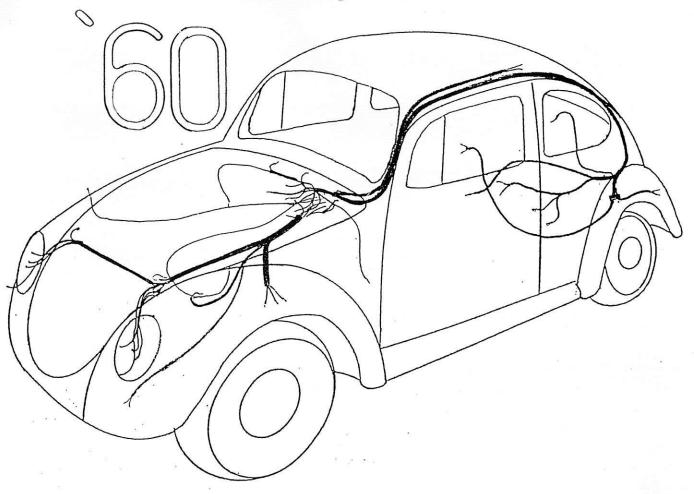
This harness kit fits 1960 Beetle hardtop sedans as shown above. Original 6 volt factory design. Can be adapted to 12 volt. Semaphore wiring not included.
