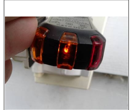
Open ground and not GFCI protected
