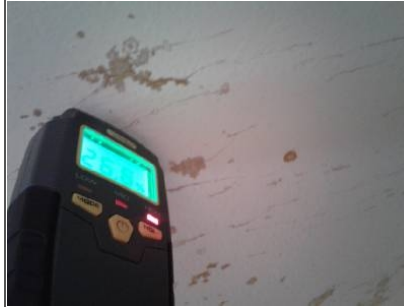
High moisture reading taken indicating active leak
