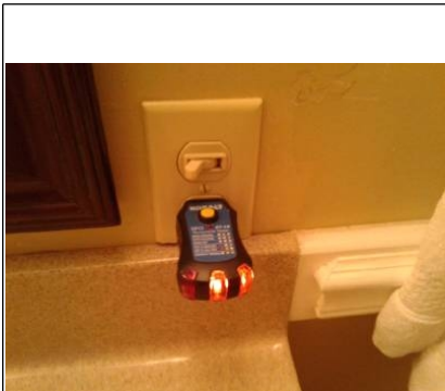
Not GFCI protected receptacle
