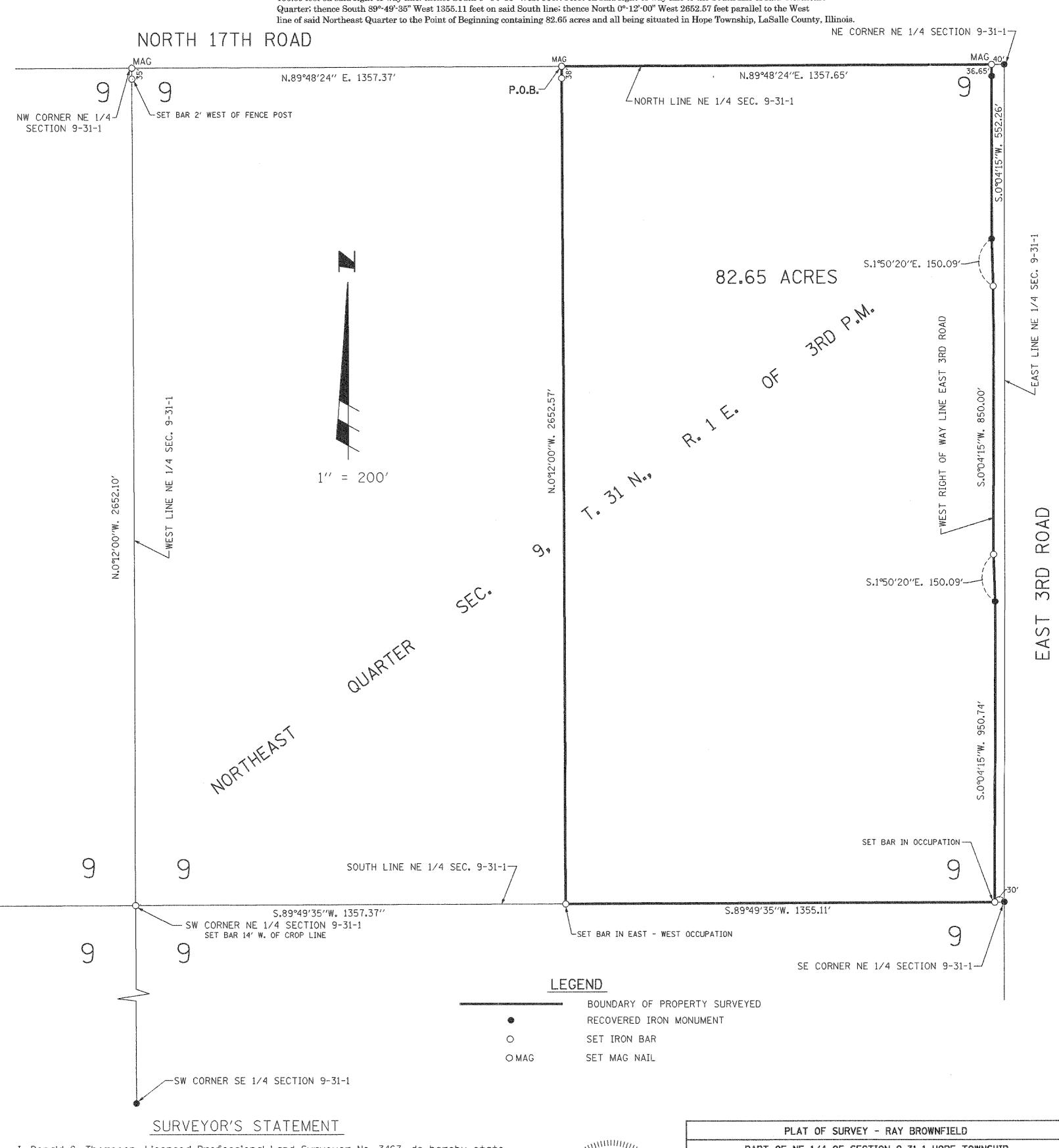
representation of a survey made under my direction for Mr. Ray Brownfield and conforms to the current Illinois minimum standards for a boundary survey. Field work was completed in February 2022 with bearings referenced to the Illinois State Plane Coordinate Systom-Fact I, Ronald C. Thompson, Licensed Professional Land Surveyor No. 3467, do hereby state in February 2022 with bearings referenced to the Illinois State Plane Coordinate System-East Zone.
