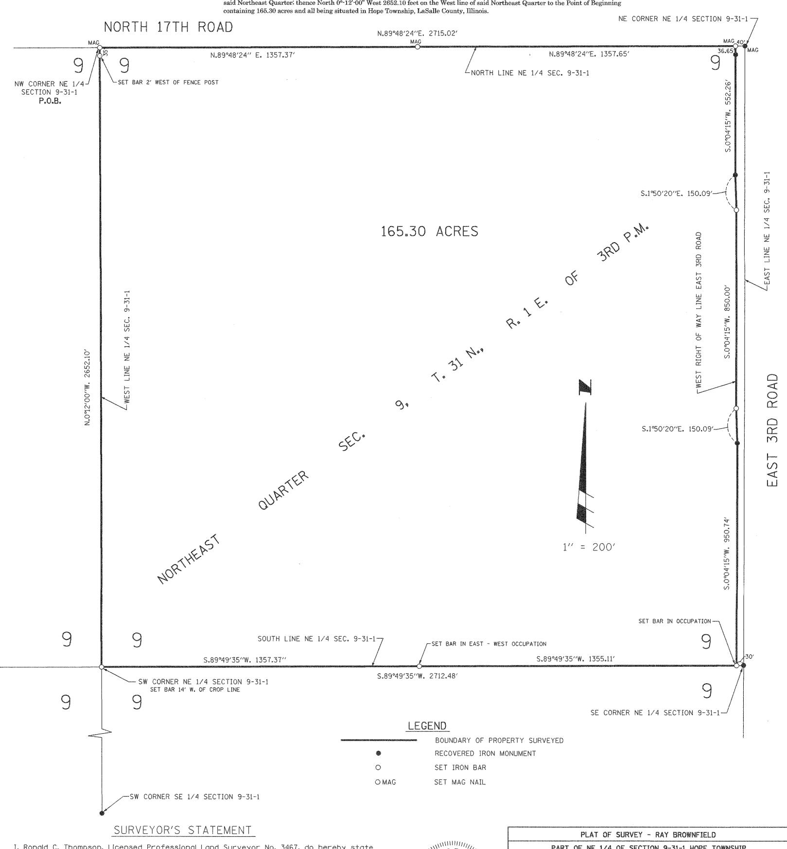
representation of a survey made under my direction for Mr. Ray Brownfield and conforms to the current Illinois minimum standards for a boundary survey. Field work was completed in February 2022 with bearings referenced to the Illinois State Plane Coordinate Survey. the current Illinois minimum standards for a boundary survey. Fleia work was completed in February 2022 with bearings referenced to the Illinois State Plane Coordinate System-East Zone.
