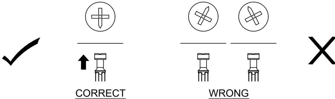
When fitting cam lock , ensure starting position is correct before you insert connecting quickfit.
