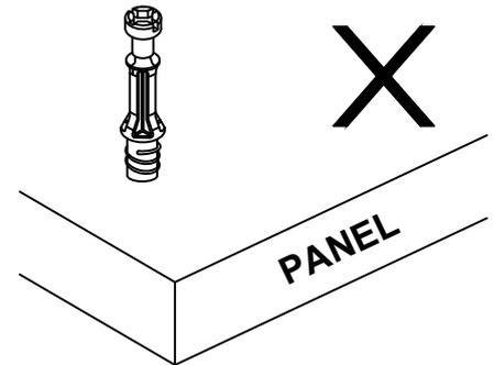
Tighten quickfit until shoulder is flush with panel . Do not overtighten or undertighten.
