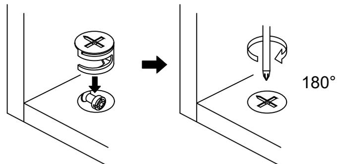
Turn cam lock clockwise to tighten.
