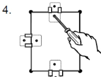
4. Screw through the patch into Repair Clips. Place screws 3/4" from the edge of the patch.
