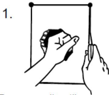
1. Draw pencil outline around the area to be removed. Cut along line and remove cut out piece.
