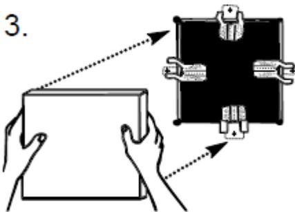
3. Cut a patch to the proper size and place in the hole.
