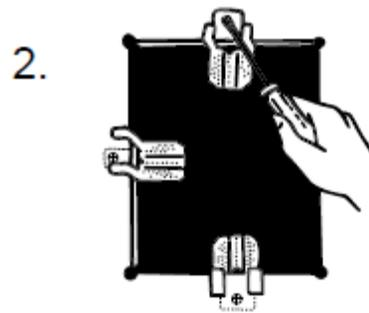
2. Place Repair Clips 6" apart around the hole. Secure with screws 3/4" from the hole edge.
