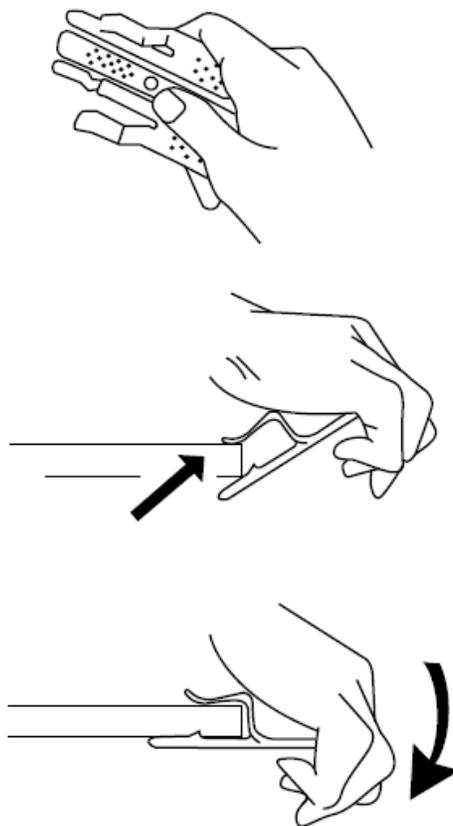
FIGURE 9—PREST-IN INSTA-BACK INSTALLATION (SECOND ILLUSTRATION)
