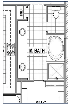
Drop in Tub at Main Bath
