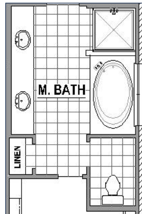
Drop in Tub at Main Bath
