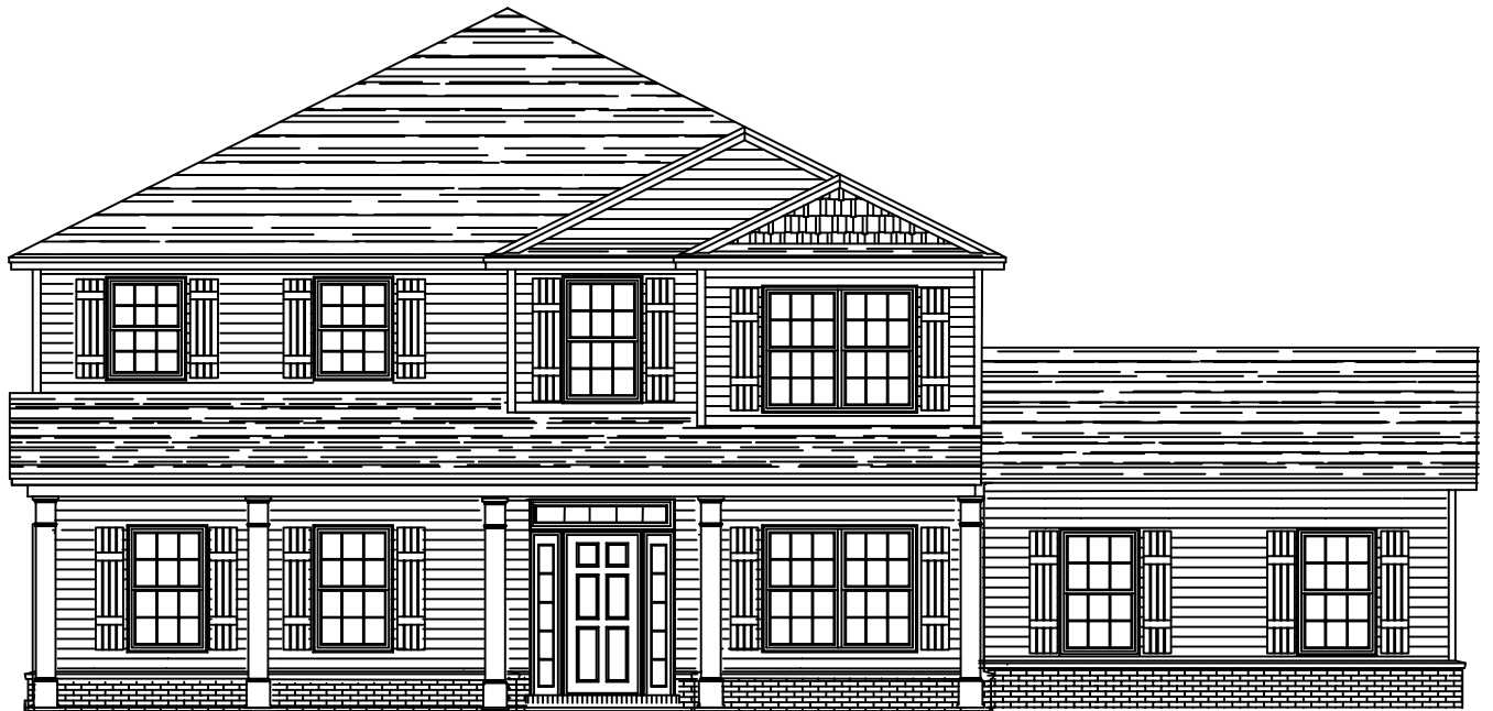
FRONT ELEVATION "B" SIDE ENTRY GARAGE
