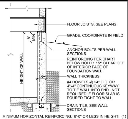
MINIMUM HORIZONTAL REINFORCING: 8'-0" OR LESS IN HEIGHT: (1) #4 BAR WITHIN 12" OF TOP OF WALL AND AT MID HEIGHT. GREATER THAN 8'-0" IN HEIGHT, PROVIDE (1) #4 BAR WITHIN 12" OF TOP OF WALL AND AT THIRD POINTS OF THE WALL
