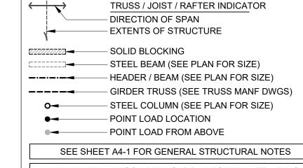
ALL LVL AND 2x WOOD BEAMS: (D) = DROPPED. (F) = FLUSH ALL HEADERS AND BEAMS TO BEAR ON MINIMUM (1) KING STUD & (1) JACK STUD EACH SIDE OF OPENING, U.N.O.
