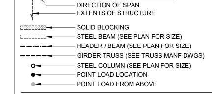
SEE SHEET A4-1 FOR GENERAL STRUCTURAL NOTES ALL LVL AND 2x WOOD BEAMS: (D) = DROPPED. (F) = FLUSH
