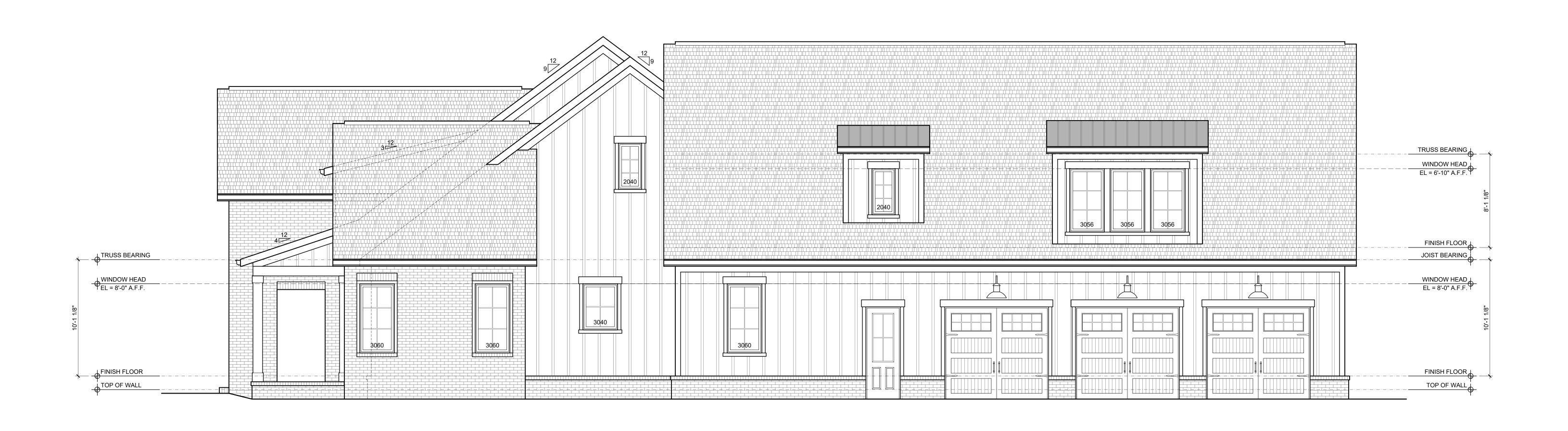
ELEVATION MATERIAL LEGEND — STANDING SEAM METAL ROOF —BOARD & BATTEN SIDING BRICK VENEER
