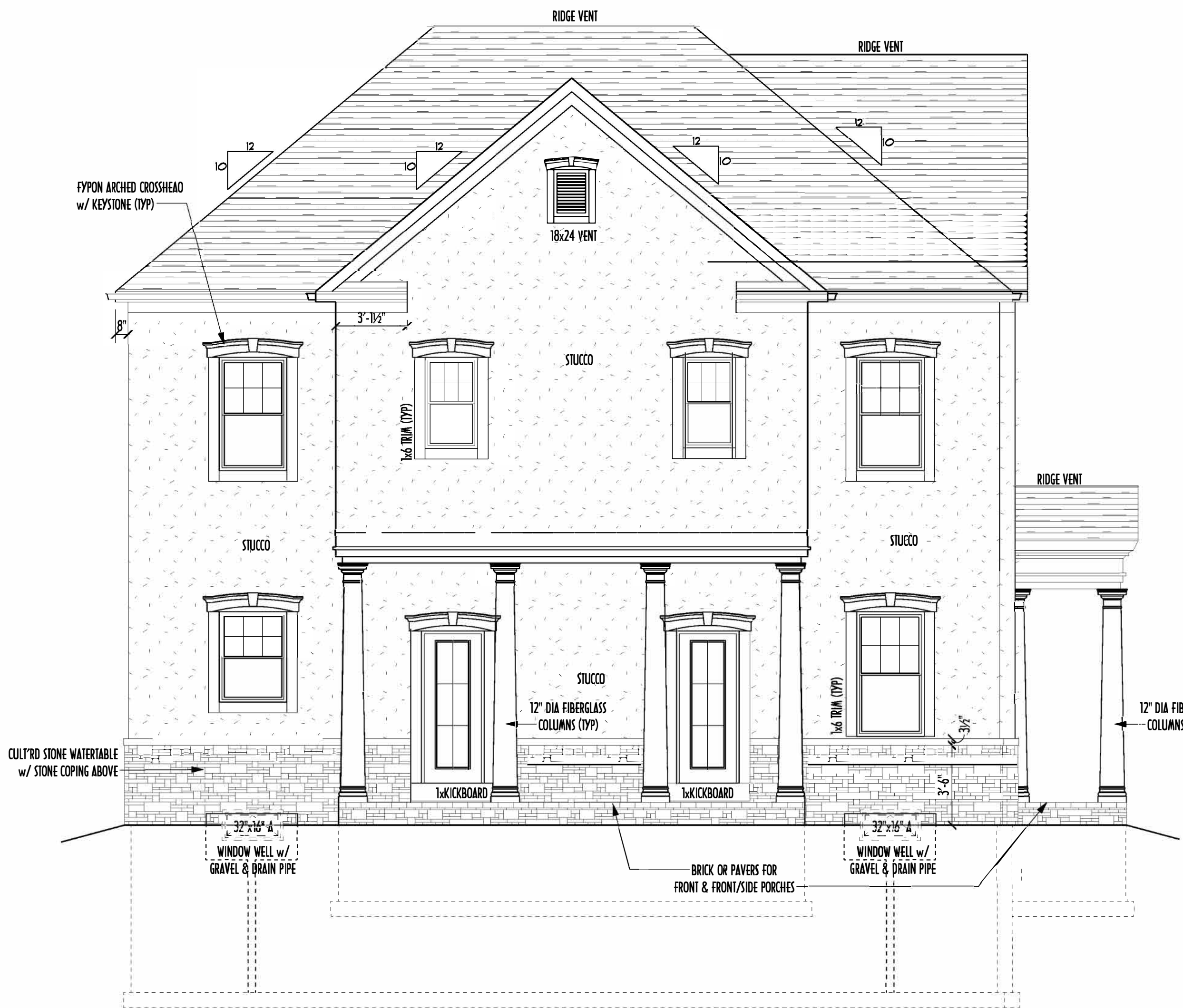
LEFT/FRONT ELEVATION (ON TARTAN RIDGE BLVD) SCALE: 1/4" = 1'-0"
