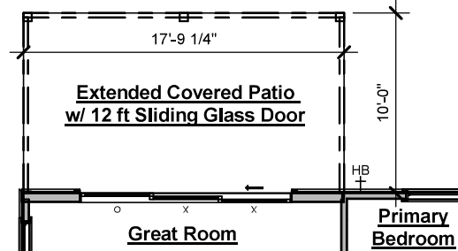
Covered Patio Extension with 12ft Sliding Glass Door
