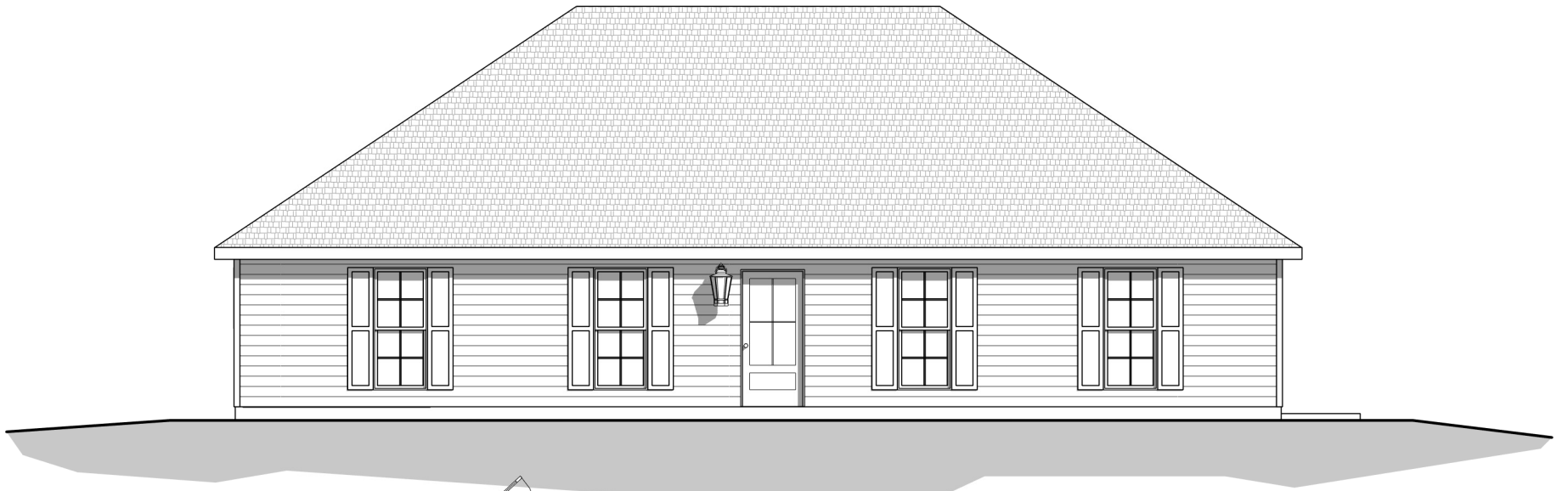
FRONT ELEVATION 8'-1" PLATE HEIGHT - 8' CLG. 10:12 ROOF PITCH
