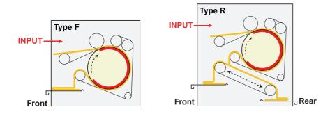
**Rear Return** allows flexibility, and increased production as additional piece processing is performed by separate receiving operators or a Skyline automatic folder
