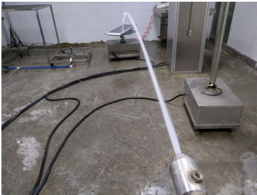
Photo 3: IPX5 test of model
