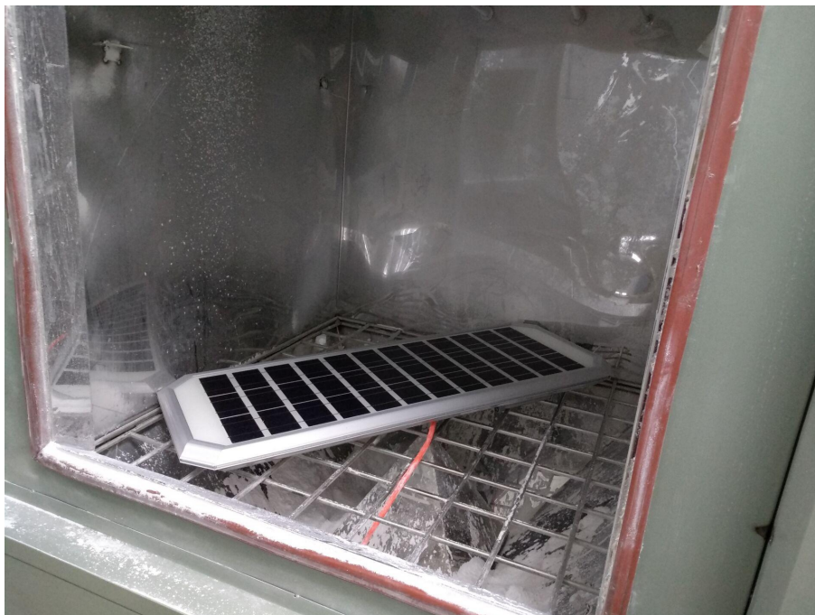
Photo 2: IP6X test of model
