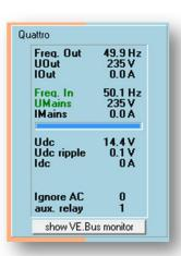
With Multi firmwares xxyy460 and up, VEConfig will indicate why the AC Input is rejected and will also show an indication of the remaining waiting time as a blue bar.
