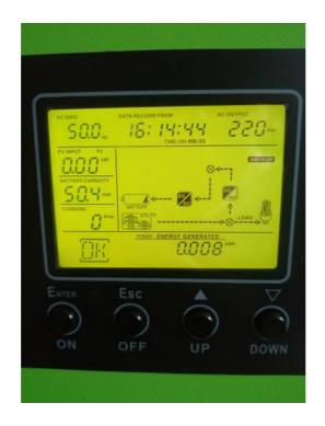
Enter and Down button to check the battery's voltage and soc. For this example, you can see voltage is 50.4V and SOC is 100%. Attention: The blank on the screen means step.
