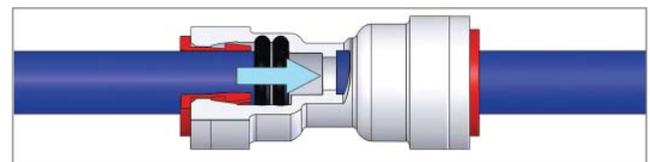
Push connect fittings are connected by firmly pushing one end of the tube into the fitting. It is important to push the tubing all the way into the fitting for a complete seal.
