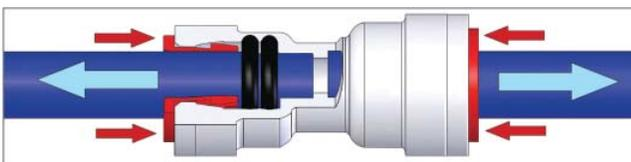
Remove the tube by holding the round retention ring tightly against the fitting then pull the tubing away from the fitting while twisting and the tubing should slowly release from the fitting.
