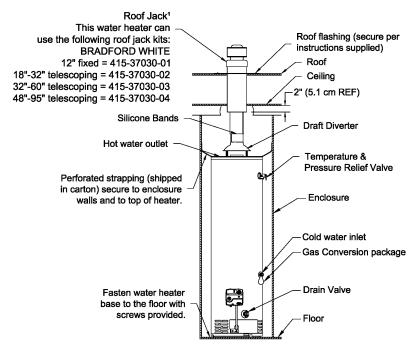
If the water heater is a new installation, then a roof jack is mandatory
