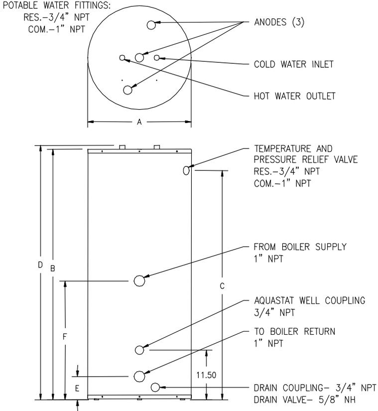
**Figure 1 – Tank Layout**
