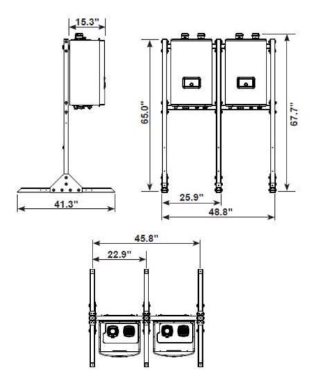
Note: Drawing shows one Base Rack, one Extension Rack, and two heaters. For back-to-back installation, rear dimensions are identical to front dimensions. When more Extension Racks are added, the width dimension of each Extension Rack is added.
