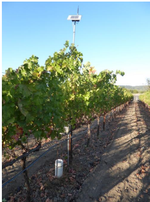
A soil moisture probe at work in a California vineyard. Photograph by Eric Pooler
