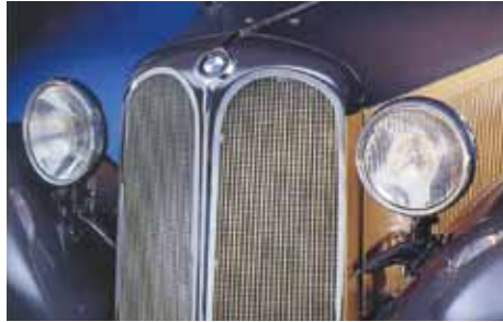
The 303 was the first BMW to feature the kidney-shaped grill and an inline six-cylinder engine.
