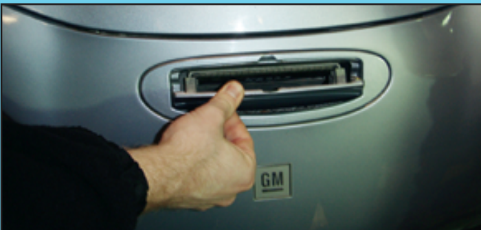
The charging receptacle of the General Motors EV1.
