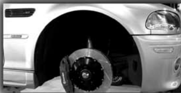
BMW M-3 Brembo brake kit & installation
