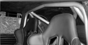
BMW 2002 Sparco DTM seats & Speedware fabricated roll bar
