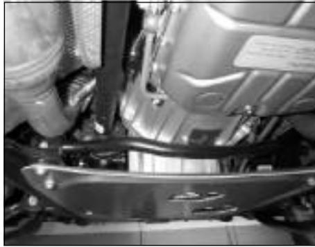
Shows driveshaft to front differential and skid plate. If you know where to look, you can see the axle passing through the oil sump.
