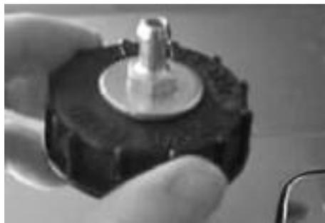
Drill a hole and enlarge it to the size of the hose fitting. Screw that baby in there and secure from the back (see picture-cap with fitting) with the brass nut. Yep, just like that. Too bad it was sunny out and the flash didn't light up the inside where I put black RTV on black plastic. You would have been real impressed with the overwhelming difficulty of the job.
