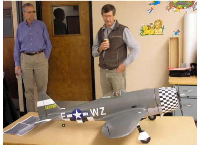
Mike Melendy – Top Flite modified ARF. Wingspan 63” Standoff scale. Engine OS.91 4-stroke.
