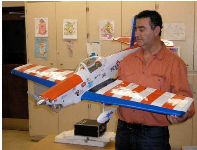
Yohay Hahamy – Carl Goldberg Super Chipmunk kit, took 55 hrs to build, modeled after plane hanging at EAA museum in Oskosh. OS.61FX with inverted muffler, light kit, 11x7 prop, Airtronics Vision radio gear.
